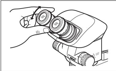
4. Set the zoom adjustment knob ① for the lowest magnification and rotate the focus adjustment knob ② to bring the specimen into approximate focus.
